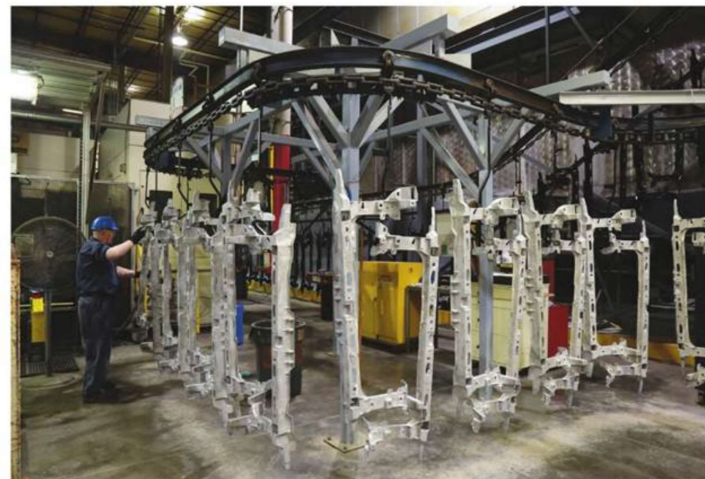
Die cast magnesium automotive front end structures such as these help manufacturers reduce vehicle weight.
