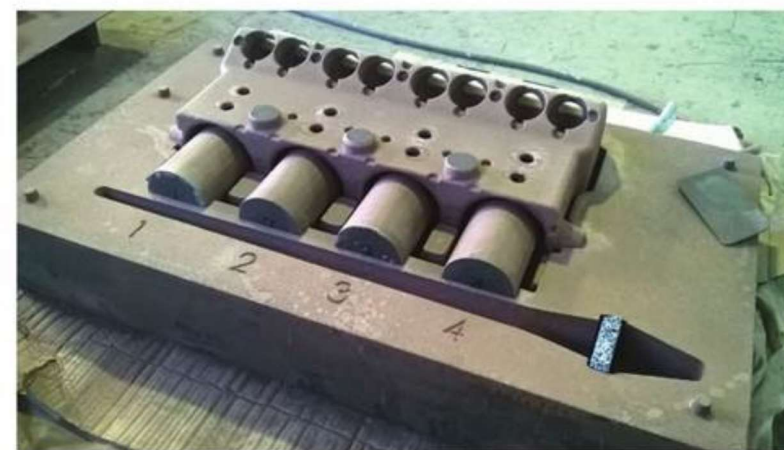
A mould produced with the Voxeljet VX1000 for an engine block casting to repair a 1914 Delage car.
