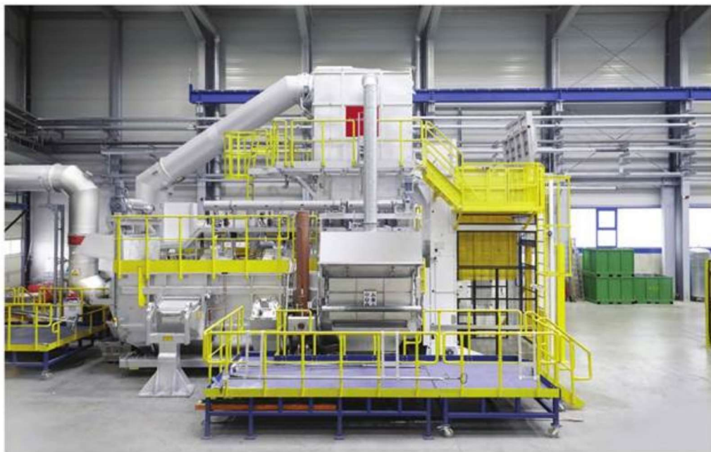
StrikoWestofen's "BigStruc" melting furnace can handle everything from complete stacks of pig iron through to small, thin-walled return material.
