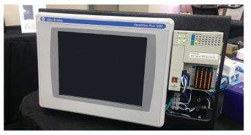
Programmable Logic Controller (PLC) PLC is a ruggedized computer used for industrial automation. These controllers can automate a specific process, machine function or an entire production line.
